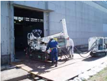
SSS type machine approaching into a building (EAZET)
